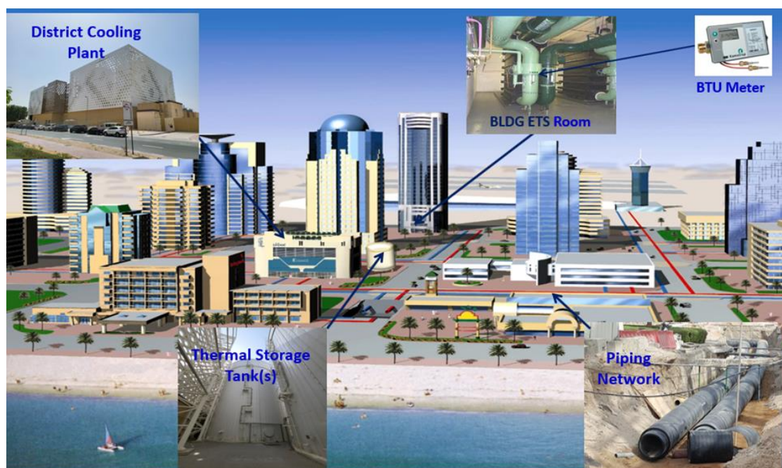
Figure 1. Typical District Cooling System
